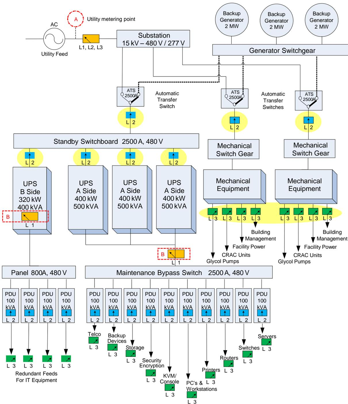
**Figure 4. Monitoring and measurement points**
