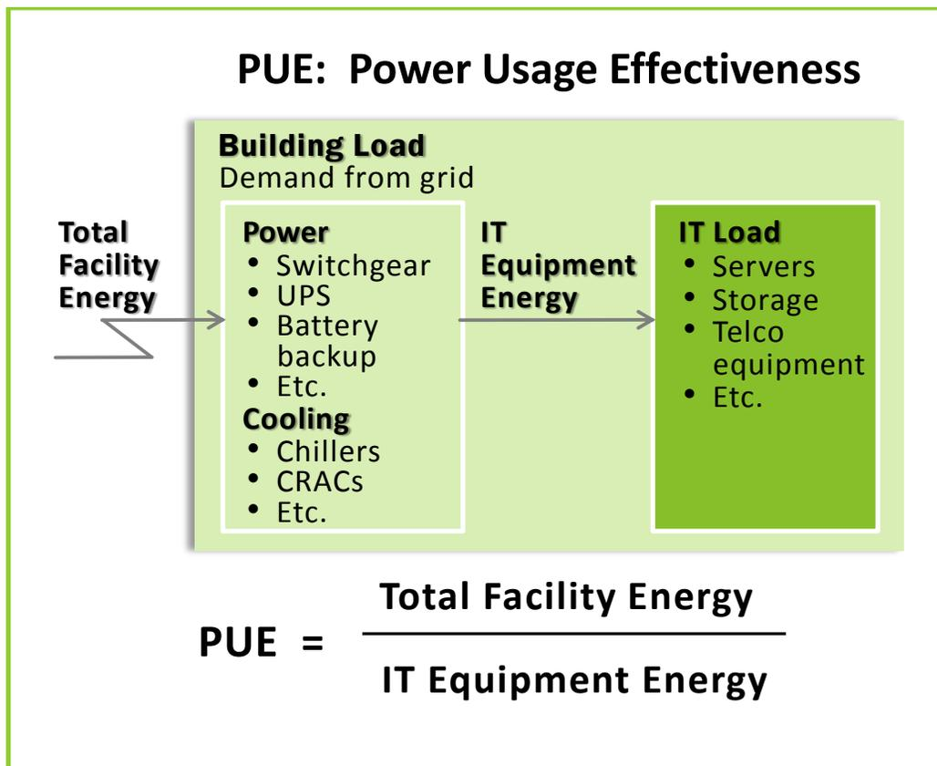
Figure 1. Illustration of how PUE would be calculated in a data center
