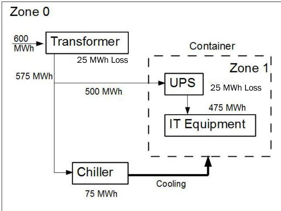
**Figure 17. Partial PUE Usage Example 1**
