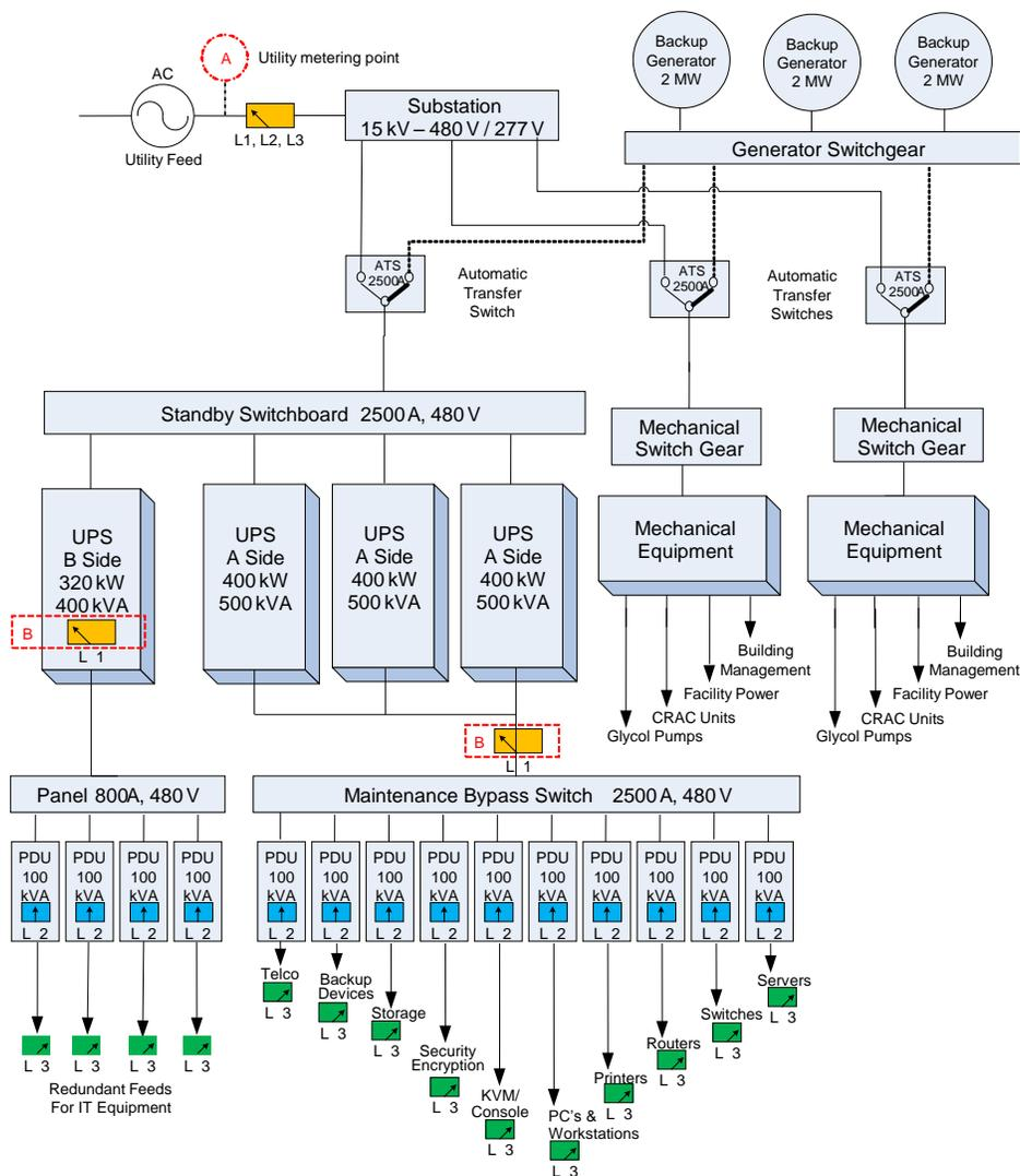
**Figure 2. Graphical representation of the three PUE measurement levels for a typical data center**
