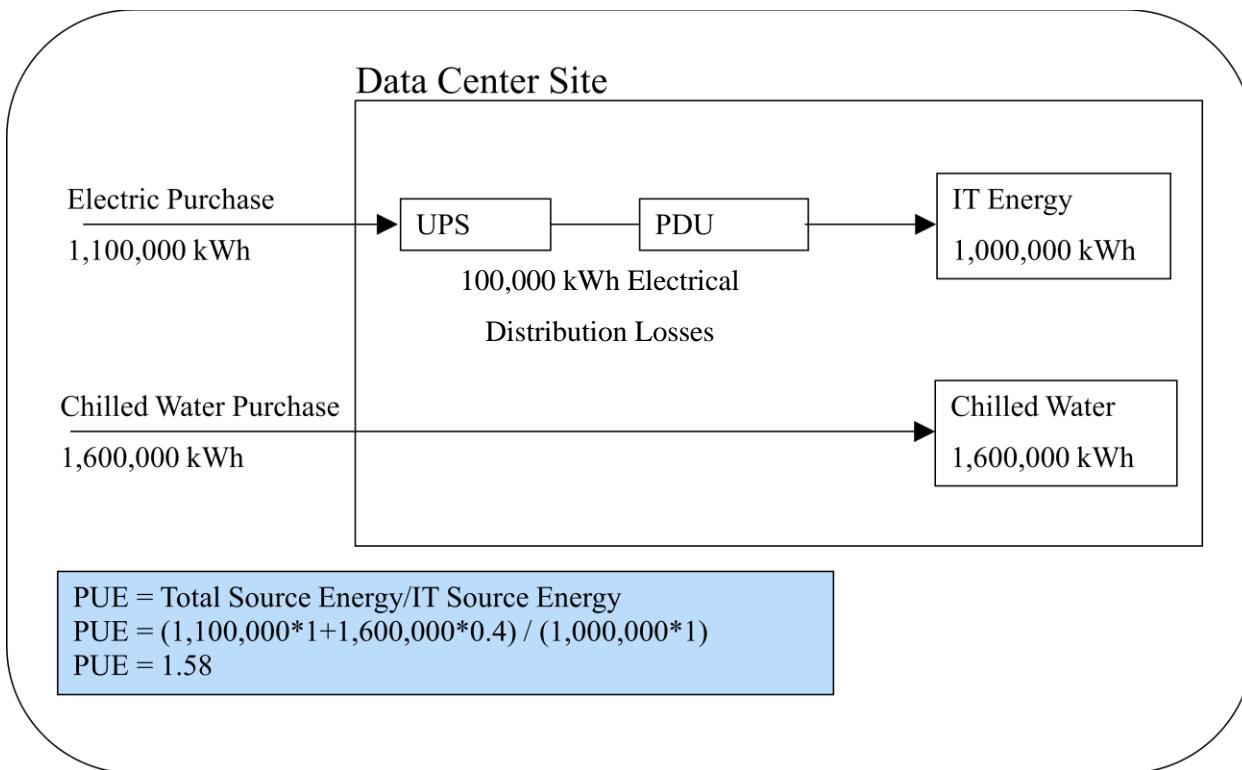
Figure 8. Example PUE calculation for a data center that purchases electricity and chilled water
