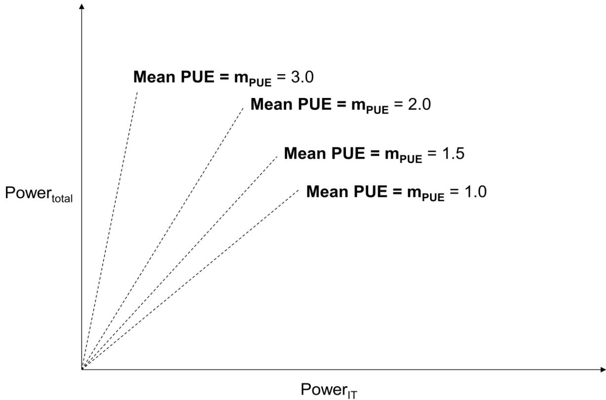
**Figure 20. Proportional data center power scalabilities at several PUE values**
