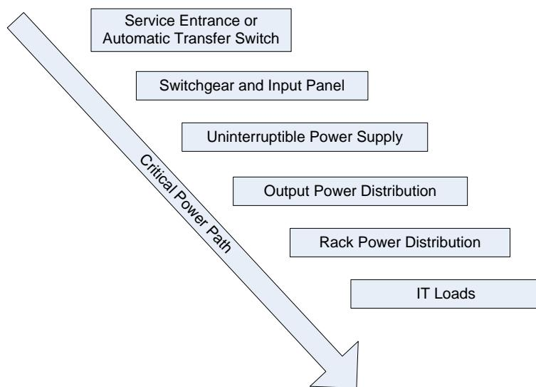
**Figure 5. Hierarchy of critical power path measurement points**
