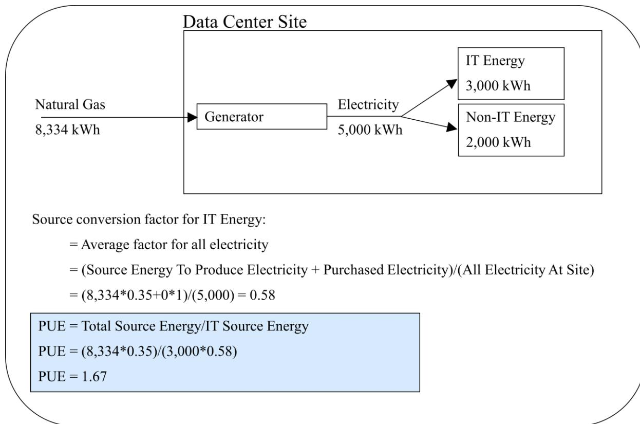
**Figure 9. Example PUE calculation for a data center that purchases natural gas**
