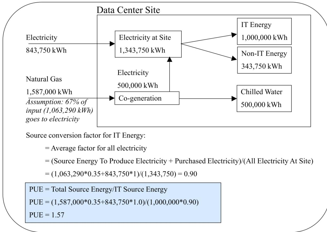
**Figure 11. Example PUE calculation for a data center with electricity and natural gas cogeneration**
