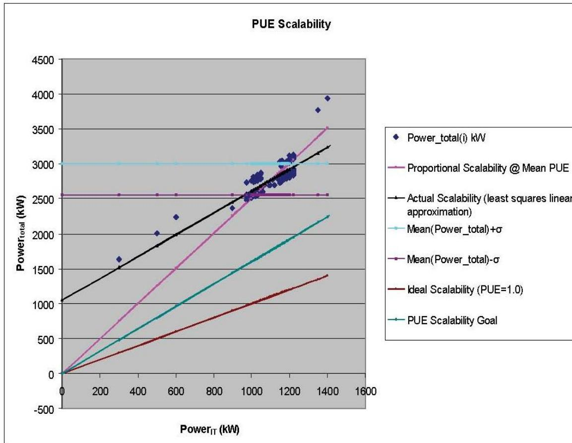
**Figure 22. Power<sub>total</sub> variations versus Power<sub>IT</sub>**
