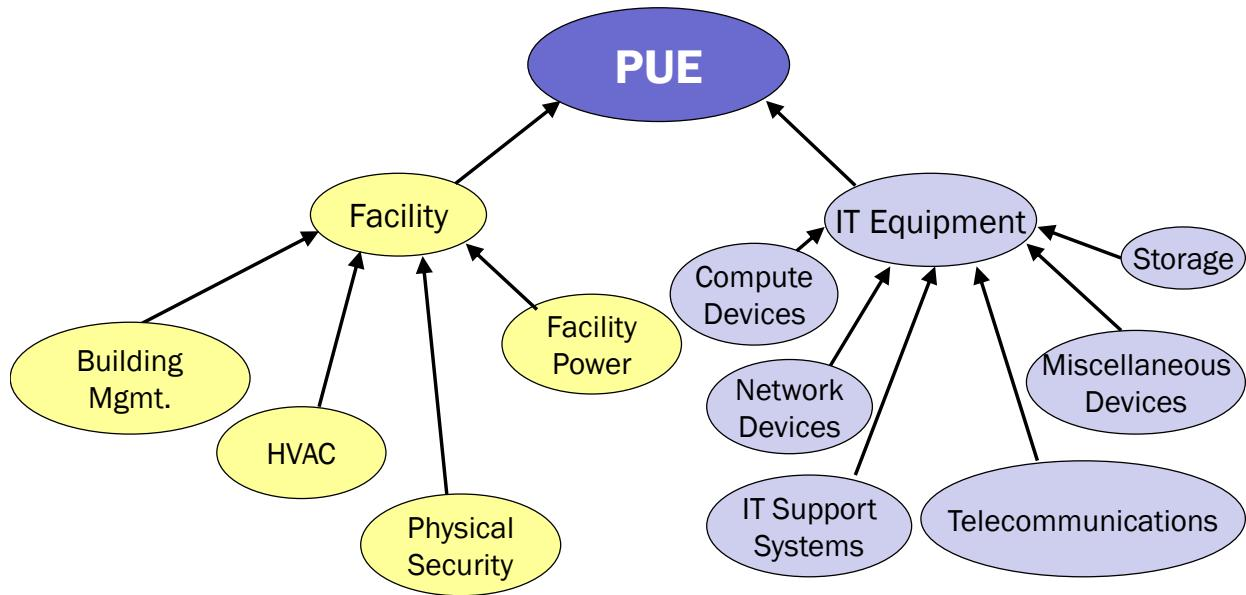
**Figure 3. Overview of the subcomponents within a typical data center's facility and IT equipment**
