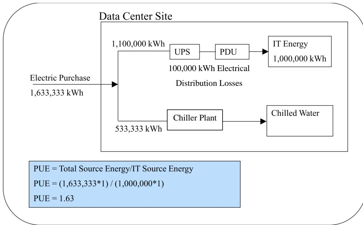
Figure 7. Example PUE calculation for a data center that purchases all electricity
