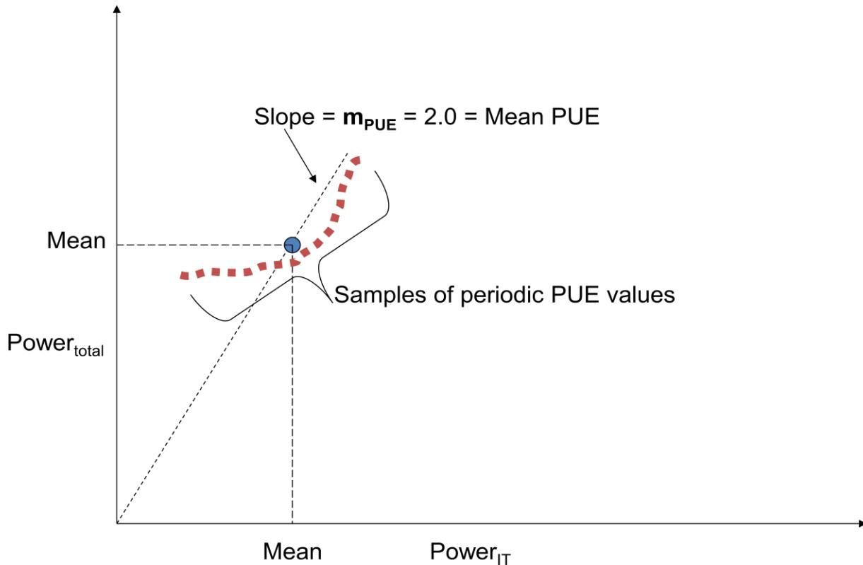
**Figure 21. Proportional power scaling in a data center with mean PUE = 2.0**
