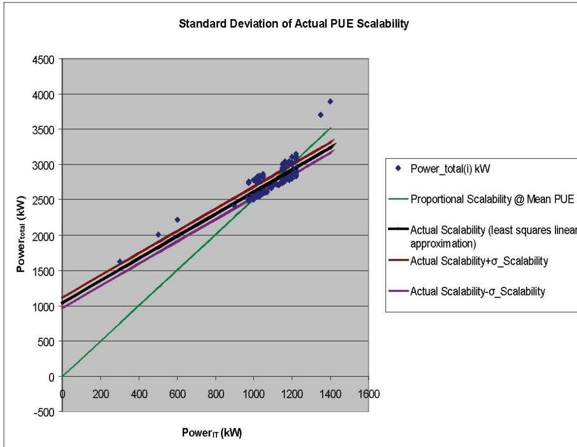
**Figure 23. Actual PUE Scalability and standard deviation of Actual PUE Scalability**
