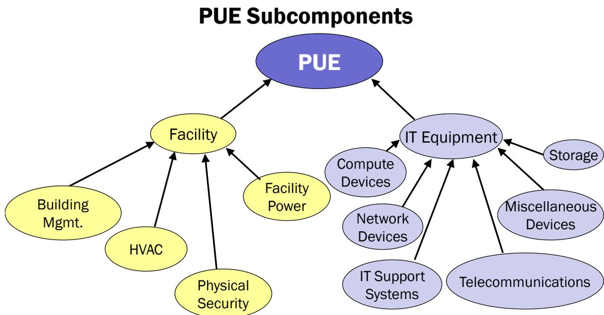
**Figure 3. Overview of the subcomponents within a typical data center's facility and IT equipment**
