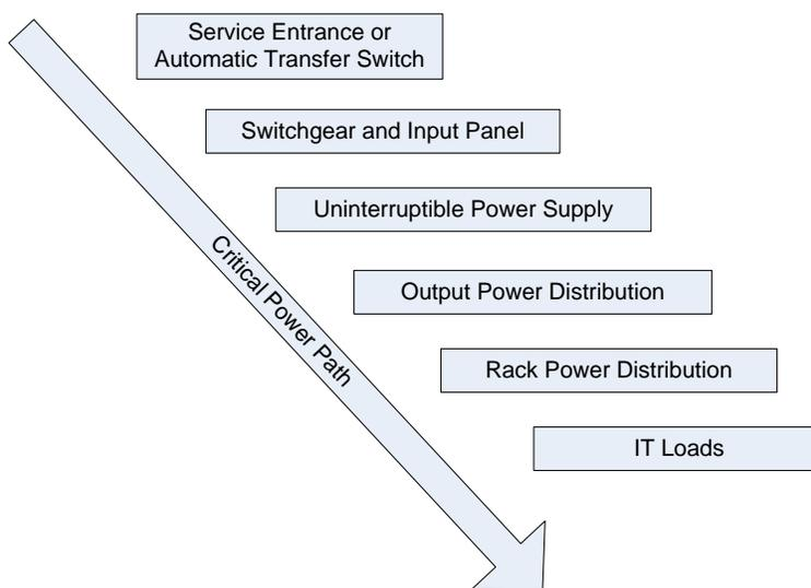
**Figure 5. Hierarchy of critical power path measurement points**
