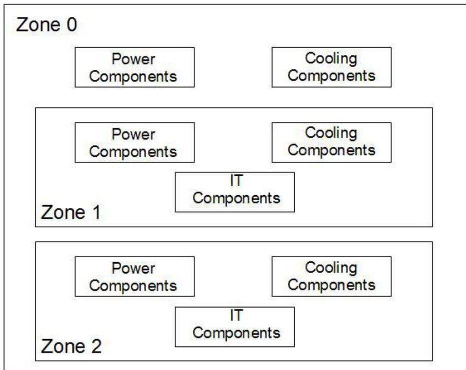
**Figure 15. Boundaries and zones in a sample data center facility**
