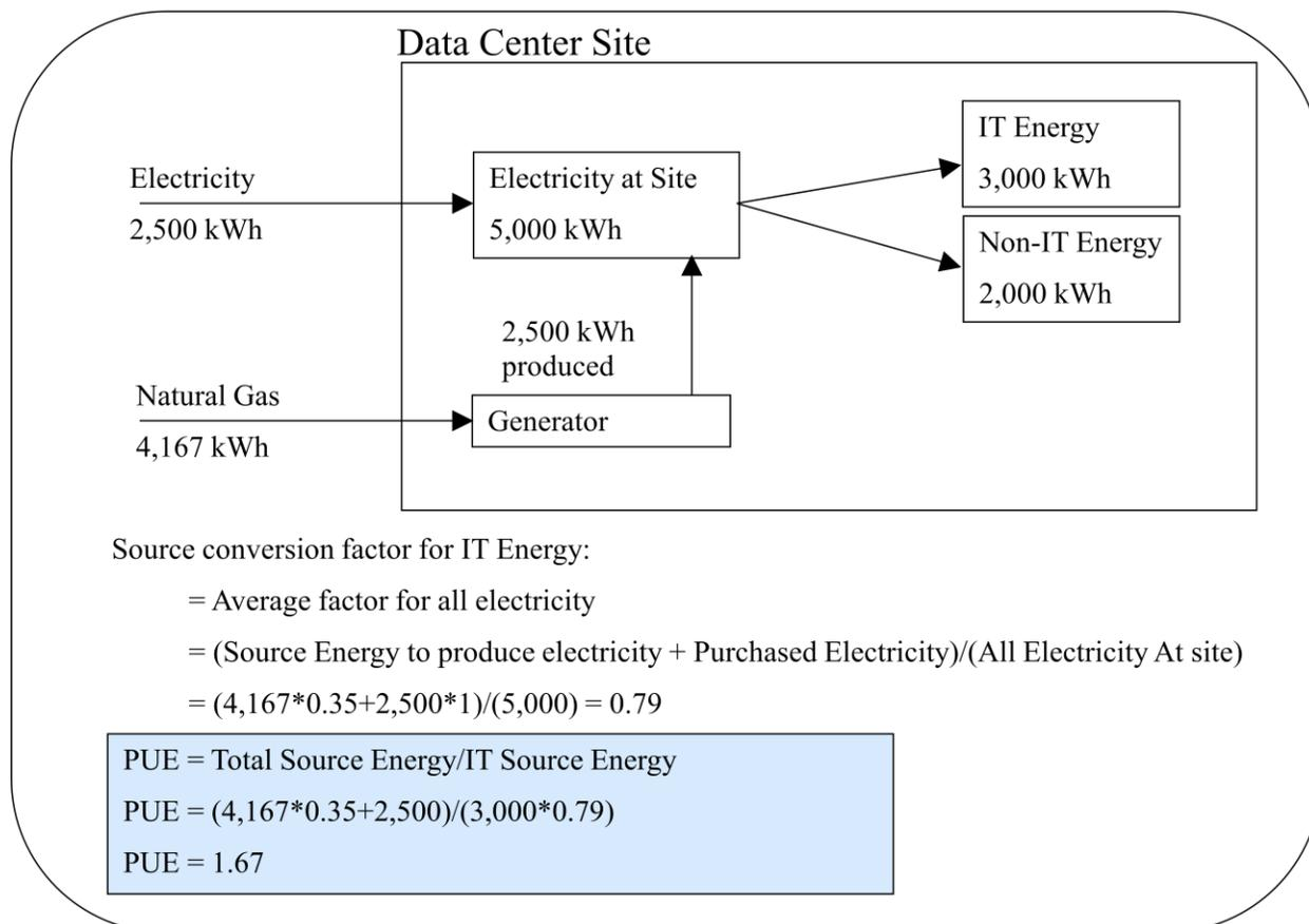
**Figure 10. Example PUE calculation for a data center that purchases electricity and natural gas**
