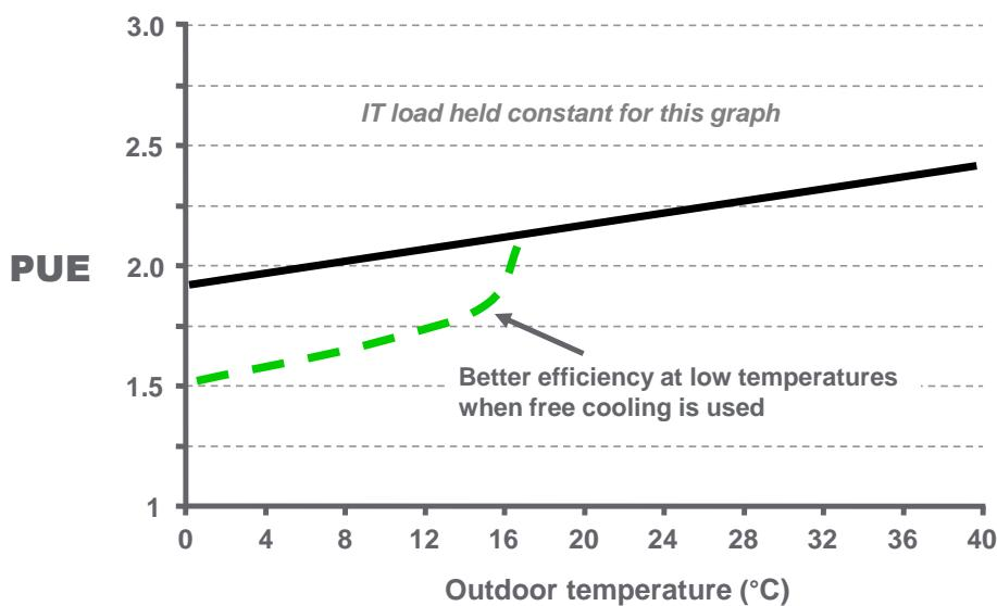
**Figure 6.** Sample illustration of the relationship between PUE and outdoor temperature
