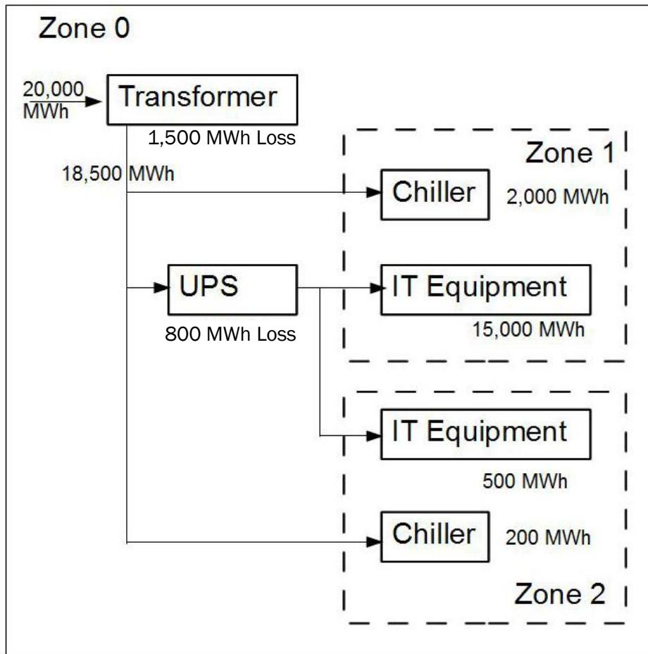
**Figure 19. Partial PUE Usage Example 3**
