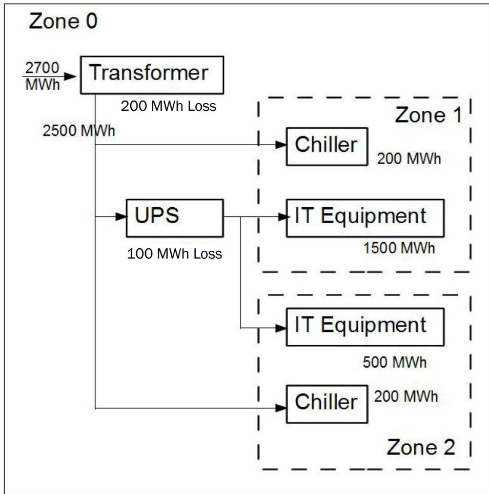
**Figure 18. Partial PUE Usage Example 2**
